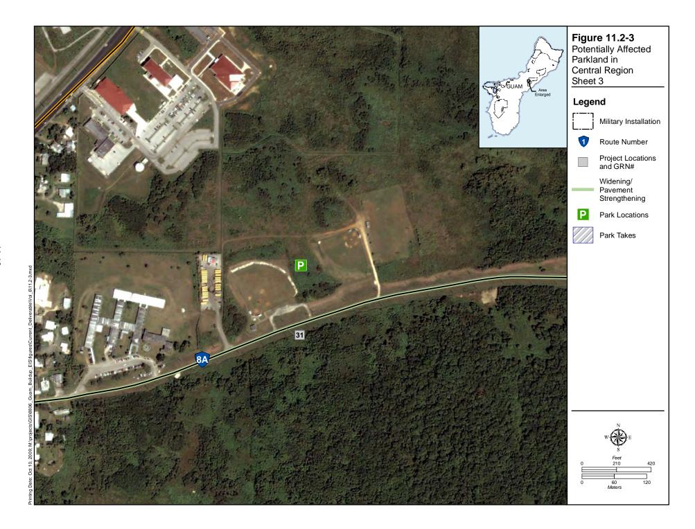
• Chinese Park would be affected by GRN #33 intersection widening at Routes 1 and 14 (see Figure 11.2-3). The existing ROW parcel line appears to indicate that the existing roadway is built partially inside the park ROW. Approximately 15,900 ft<sup>2</sup> or 0.36-ac (0.15-ha) of land would need to be acquired to correct this situation and to allow the intersection improvements.
